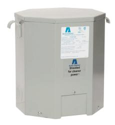
ACME general purpose transformer, encapsulated core, 7.5 kVA, 1-phase, 190/200/208/220 or 380/400/416/440 VAC primary, 120/240 VAC secondary, 50/60 Hz, electrostatic shield, NEMA 3R, wall mount.
