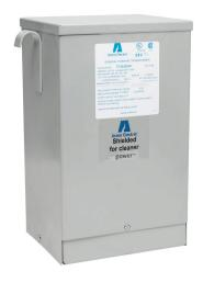
ACME general purpose transformer, encapsulated core, 5 kVA, 1-phase, 190/200/208/220 or 380/400/416/440 VAC primary, 120/240 VAC secondary, 50/60 Hz, electrostatic shield, NEMA 3R, wall mount.
