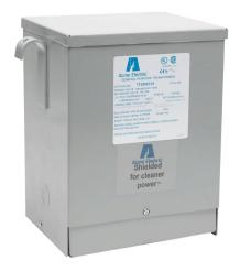
ACME general purpose transformer, encapsulated core, 3 kVA, 1-phase, 190/200/208/220 or 380/400/416/440 VAC primary, 120/240 VAC secondary, 50/60 Hz, electrostatic shield, NEMA 3R, wall mount.
