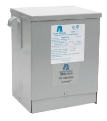
ACME general purpose transformer, encapsulated core, 3 kVA, 1-phase, 190/200/208/220 or 380/400/416/440 VAC primary, 120/240 VAC secondary, 50/60 Hz, electrostatic shield, NEMA 3R, wall mount.
