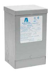
ACME general purpose transformer, encapsulated core, 1 kVA, 1-phase, 190/200/208/220 or 380/400/416/440 VAC primary, 120/240 VAC secondary, 50/60 Hz, electrostatic shield, NEMA 3R, wall mount.
