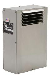
Stratus CFC-free air-to-air heat exchanger, 44 W/deg C (24 W/ deg F), 120 VAC operating voltage, 50/60 Hz, 0.37A running current, side mount, 304 stainless steel. For use with NEMA/UL Type 4X enclosures.
