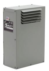
Stratus CFC-free air-to-air heat exchanger, 44 W/deg C (24 W/ deg F), 120 VAC operating voltage, 50/60 Hz, 0.37A running current, side mount, cold-rolled steel, ANSI 61 gray, powder coat finish. For use with NEMA/UL Type 4 enclosures.
