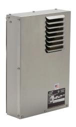
Stratus CFC-free air-to-air heat exchanger, 22 W/deg C (12 W/deg F), 24 VDC operating voltage, 0.80A running current, side mount, 304 stainless steel. For use with NEMA/UL Type 4X enclosures.
