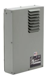
Stratus CFC-free air-to-air heat exchanger, 22 W/deg C (12 W/deg F), 24 VDC operating voltage, 0.80A running current, side mount, cold-rolled steel, ANSI 61 gray, powder coat finish. For use with NEMA/UL Type 4 enclosures.
