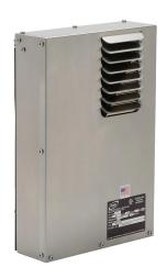
Stratus CFC-free air-to-air heat exchanger, 22 W/deg C (12 W/deg F), 120 VAC operating voltage, 50/60 Hz, 0.37A running current, side mount, 304 stainless steel. For use with NEMA/UL Type 4X enclosures.
