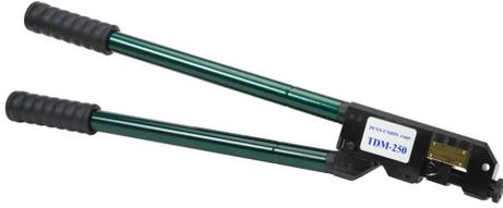
Penn-Union crimping tool, indent profile, 8 AWG-250 MCM copper and 8-4AWG aluminum capacity, compatible with Penn-Union BLU series copper compression lugs.
