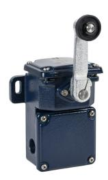
Schmersal heavy duty limit switch, side rotary lever with plastic roller, (1) N.O./(1) N.C. left and (1) N.O./(1) N.C. right contact(s), slow action, 122mm hole spacing, cast iron, (2) M25 x 1.5 cable entry.
