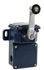
Schmersal heavy duty limit switch, side rotary lever with metal roller, (2) N.C. left and (2) N.C. right contact(s), slow action, 122mm hole spacing, cast iron, (2) M25 x 1.5 cable entry.
