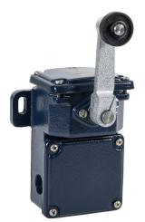
Schmersal heavy duty limit switch, side rotary lever with plastic roller, (2) N.C. contact(s), slow action, 122mm hole spacing, cast iron, (2) M25 x 1.5 cable entry.
