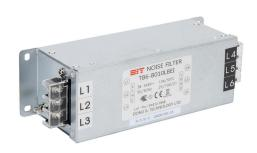
LS Electric EMI input filter, 440 VAC, 3-phase, 10A, panel mount, EMI/RFI filtering, drive rated, standard performance, screw terminals. For use with 1-phase or 3-phase AC drives.
