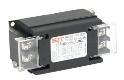
LS Electric EMI input filter, 250 VAC, 1-phase, 10A, panel mount, EMI/RFI filtering, 2-stage, drive rated, standard performance, screw terminals. For use with 1-phase AC drives.
