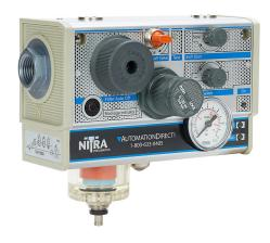
NITRA pneumatic total air prep unit, 1/2in female NPT inlet(s), 1/2in female NPT outlet(s), 7-116 psi (0.5-8 bar) adjustable range, Rynite (PET) bowl, semi-automatic drain, clog indicator, manual shutoff valve, soft start valve, pressure switch.
