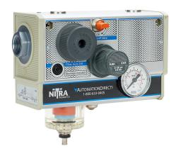
NITRA pneumatic total air prep unit, 1/2in female NPT inlet(s), 1/2in female NPT outlet(s), 7-116 psi (0.5-8 bar) adjustable range, Rynite (PET) bowl, semi-automatic drain, clog indicator, manual shutoff valve.
