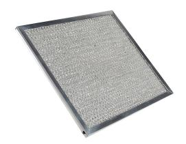
Stratus filter, replacement, 11.00 x 9.00in, 250 micron expanded aluminum, aluminum frame, washable, 60% filter efficiency. For use with 2000 BTU/H TA20 series enclosure air conditioners.
