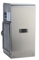
Stratus air conditioner, 2705 BTU/H, R-134a, 230 VAC operating voltage, 304 stainless steel housing, side mount. For use with NEMA/UL Type 4X enclosures.
