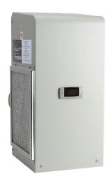
Stratus air conditioner, 2705 BTU/H, R-134a, 230 VAC operating voltage, carbon steel housing, ANSI 61 gray, side mount. For use with NEMA/UL Type 12 enclosures.
