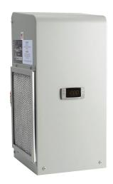
Stratus air conditioner, 2705 BTU/H, R-134a, 230 VAC operating voltage, carbon steel housing, ANSI 61 gray, side mount. For use with NEMA/UL Type 4 enclosures.
