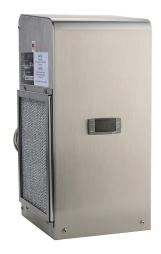
Stratus air conditioner, 2705 BTU/H, R-134a, 115 VAC operating voltage, 304 stainless steel housing, side mount. For use with NEMA/UL Type 4X enclosures.
