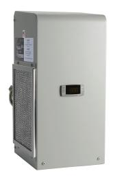
Stratus air conditioner, 2705 BTU/H, R-134a, 115 VAC operating voltage, carbon steel housing, ANSI 61 gray, side mount. For use with NEMA/UL Type 4 enclosures.
