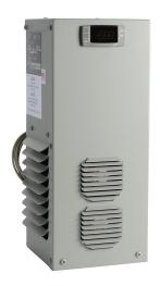
Stratus air conditioner, 1500 BTU/H, R-134a, 48 VDC operating voltage, carbon steel housing, ANSI 61 gray, filter-free, side mount. For use with NEMA/UL Type 4 enclosures.
