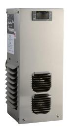
Stratus air conditioner, 1690 BTU/H, R-134a, 115 VAC operating voltage, 304 stainless steel housing, filter-free, side mount. For use with NEMA/UL Type 4X enclosures.
