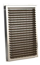
Stratus filter and louvered frame assembly, 16.30 x 10.30in, 250 micron stainless steel mesh, 304 stainless steel frame, washable, 97% filter efficiency. For use with 5000-6000 BTU/H TA10 series enclosure air conditioners on NEMA 4X enclosures.
