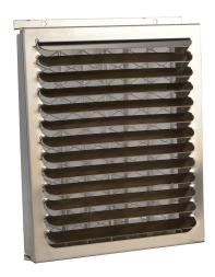
Stratus filter and louvered frame assembly, 11.30 x 7.30in, 250 micron stainless steel mesh, 304 stainless steel frame, washable, 97% filter efficiency. For use with 2000-4000 BTU/H TA10 series enclosure air conditioners on NEMA 4X enclosures.
