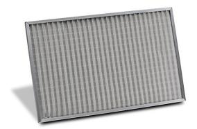
Stratus filter, replacement, 16.30 x 10.30in, 250 micron expanded aluminum, aluminum frame, washable, 60% filter efficiency. For use with 5000-6000 BTU/H TA10 series enclosure air conditioners.
