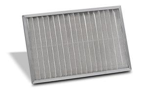
Stratus filter, replacement, 11.30 x 7.30in, 250 micron expanded aluminum, aluminum frame, washable, 60% filter efficiency. For use with 2000-4000 BTU/H TA10 series enclosure air conditioners.
