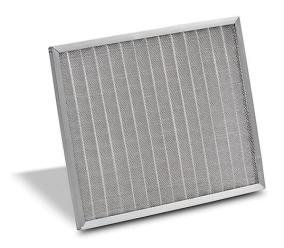
Stratus filter, replacement, 9.00 x 7.50in, 250 micron expanded aluminum, aluminum frame, washable, 60% filter efficiency. For use with 1000-1500 BTU/H TA10 series enclosure air conditioners.
