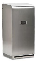
Stratus air conditioner, 1725 BTU/H, R-134a, 230 VAC operating voltage, 304 stainless steel housing, side mount. For use with NEMA/UL Type 4X enclosures.
