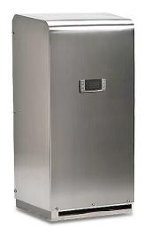
Stratus air conditioner, 1725 BTU/H, R-134a, 115 VAC operating voltage, 304 stainless steel housing, side mount. For use with NEMA/UL Type 4X enclosures.
