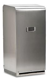
Stratus air conditioner, 1725 BTU/H, R-134a, 115 VAC operating voltage, 304 stainless steel housing, side mount. For use with NEMA/UL Type 4X enclosures.
