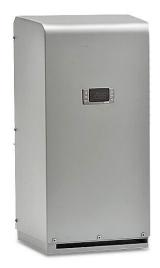
Stratus air conditioner, 1480 BTU/H, R-134a, 230 VAC operating voltage, carbon steel housing, ANSI 61 gray, side mount. For use with NEMA/UL Type 12 enclosures.
