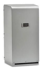
Stratus air conditioner, 1480 BTU/H, R-134a, 230 VAC operating voltage, carbon steel housing, ANSI 61 gray, side mount. For use with NEMA/UL Type 4 enclosures.
