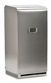
Stratus air conditioner, 1480 BTU/H, R-134a, 115 VAC operating voltage, 304 stainless steel housing, side mount. For use with NEMA/UL Type 4X enclosures.
