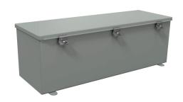
Wiegmann wiring trough, 8 x 8 x 24in (HxDxL), NEMA 4, carbon steel, ANSI 61 gray, powder coat finish, single-door.
