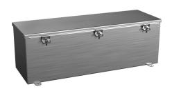
Wiegmann wiring trough, 8 x 8 x 24in (HxDxL), NEMA 1/4/4X/12, 304 stainless steel, No. 3 intermediate polished finish, single-door.
