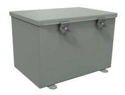
Wiegmann wiring trough, 8 x 8 x 12in (HxDxL), NEMA 4, carbon steel, ANSI 61 gray, powder coat finish, single-door.
