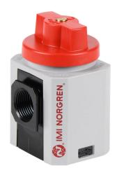
Norgren shut-off valve, 3-port (3-way), 2-position, twist, N.C., 3/4in female NPT inlet(s), 3/4in female NPT outlet(s), G1/4 female BSPP exhaust(s). For use with Excelon 84 series components.
