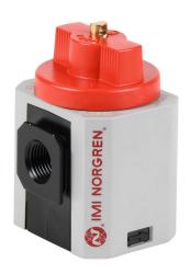
Norgren shut-off valve, 3-port (3-way), 2-position, twist, N.C., 1/2in female NPT inlet(s), 1/2in female NPT outlet(s), G1/4 female BSPP exhaust(s). For use with Excelon 84 series components.
