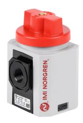
Norgren shut-off valve, 3-port (3-way), 2-position, twist, N.C., 3/8in female NPT inlet(s), 3/8in female NPT outlet(s), G1/4 female BSPP exhaust(s). For use with Excelon 84 series components.
