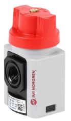
Norgren shut-off valve, 3-port (3-way), 2-position, twist, N.C., 3/8in female NPT inlet(s), 3/8in female NPT outlet(s), 1/4in female NPT exhaust(s). For use with Excelon 82 series components.
