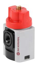
Norgren shut-off valve, 3-port (3-way), 2-position, twist, N.C., 1/4in female NPT inlet(s), 1/4in female NPT outlet(s), 1/4in female NPT exhaust(s). For use with Excelon 82 series components.
