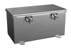
Wiegmann wiring trough, 6 x 6 x 12in (HxDxL), NEMA 1/4/4X/12, 304 stainless steel, No. 3 intermediate polished finish, single-door.
