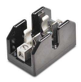
Bussmann fuse block, accepts T fuses, 60A, 600V, 1-pole, 14-2 AWG copper or aluminum, box lug, panel mount.
