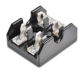
Bussmann fuse block, accepts T fuses, 30A, 600V, 2-pole, 18-10 AWG copper only, screw with pressure plate, panel mount.
