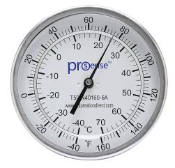
ProSense bi-metal dial thermometer, 5in diameter, 6in insertion length, -40 to 160 deg F/-40 to 70 deg C, 1/2in male NPT process connection, center back, adjustable angle mount.
