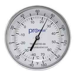
ProSense bi-metal dial thermometer, 5in diameter, 6in insertion length, -40 to 160 deg F/-40 to 70 deg C, 1/2in male NPT process connection, center back, adjustable angle mount.
