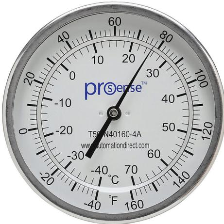
ProSense bi-metal dial thermometer, 5in diameter, 4in insertion length, -40 to 160 deg F/-40 to 70 deg C, 1/2in male NPT process connection, center back, adjustable angle mount.
