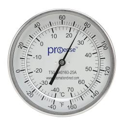
ProSense bi-metal dial thermometer, 5in diameter, 2-1/2in insertion length, -40 to 160 deg F/-40 to 70 deg C, 1/2in male NPT process connection, center back, adjustable angle mount.
