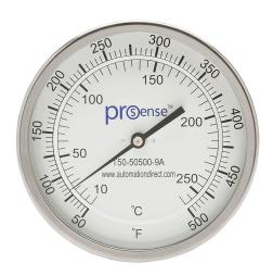
ProSense bi-metal dial thermometer, 5in diameter, 9in insertion length, 50 to 500 deg F/10 to 260 deg C, 1/2in male NPT process connection, center back, adjustable angle mount.
